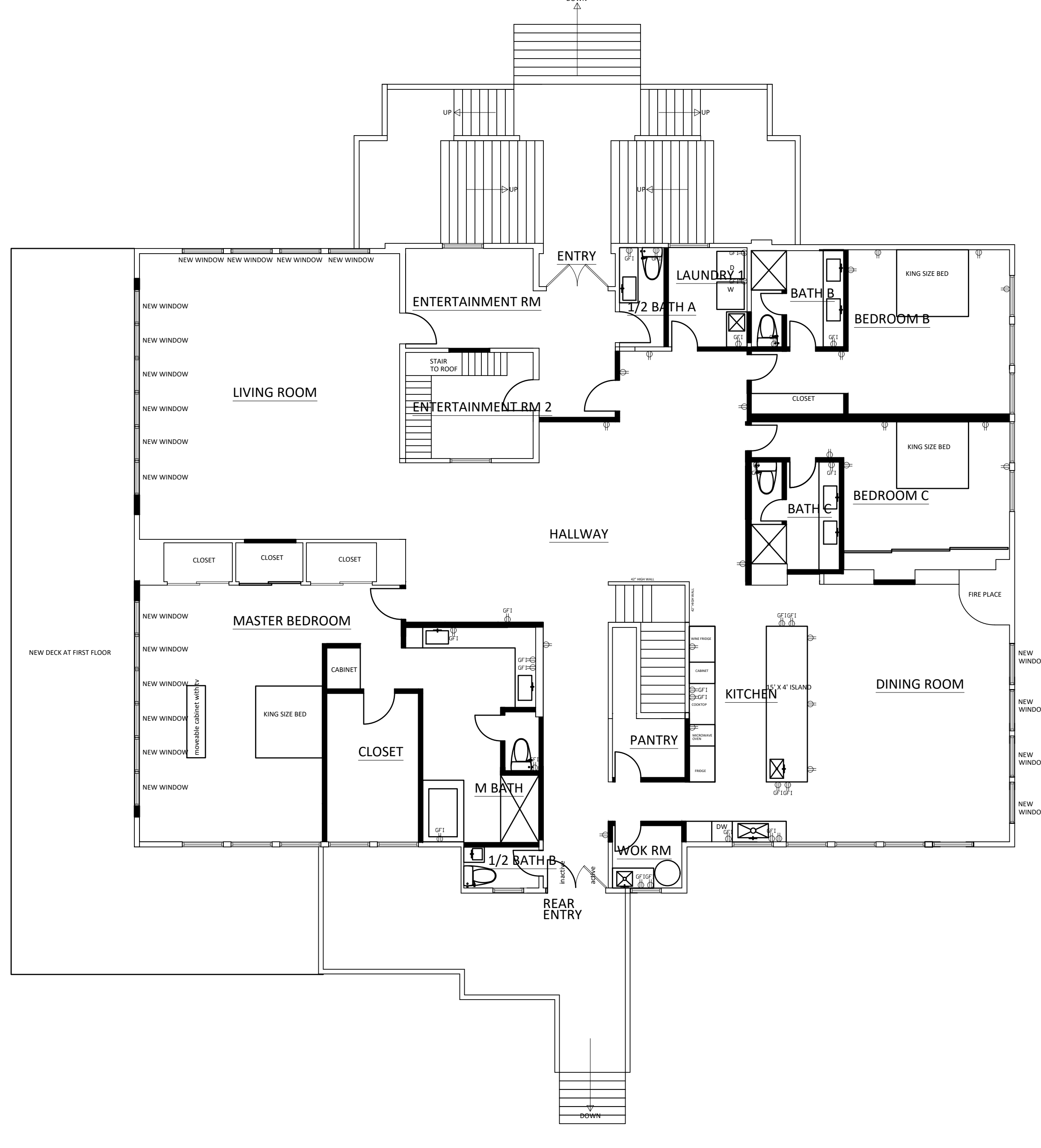
2 PROPOSED SECOND FLOOR PLAN SCALE: 1/8" = 1'-0" 0' 4' 8' 16' (NO CHANGE OF BUILDING FOOTPRINT)
