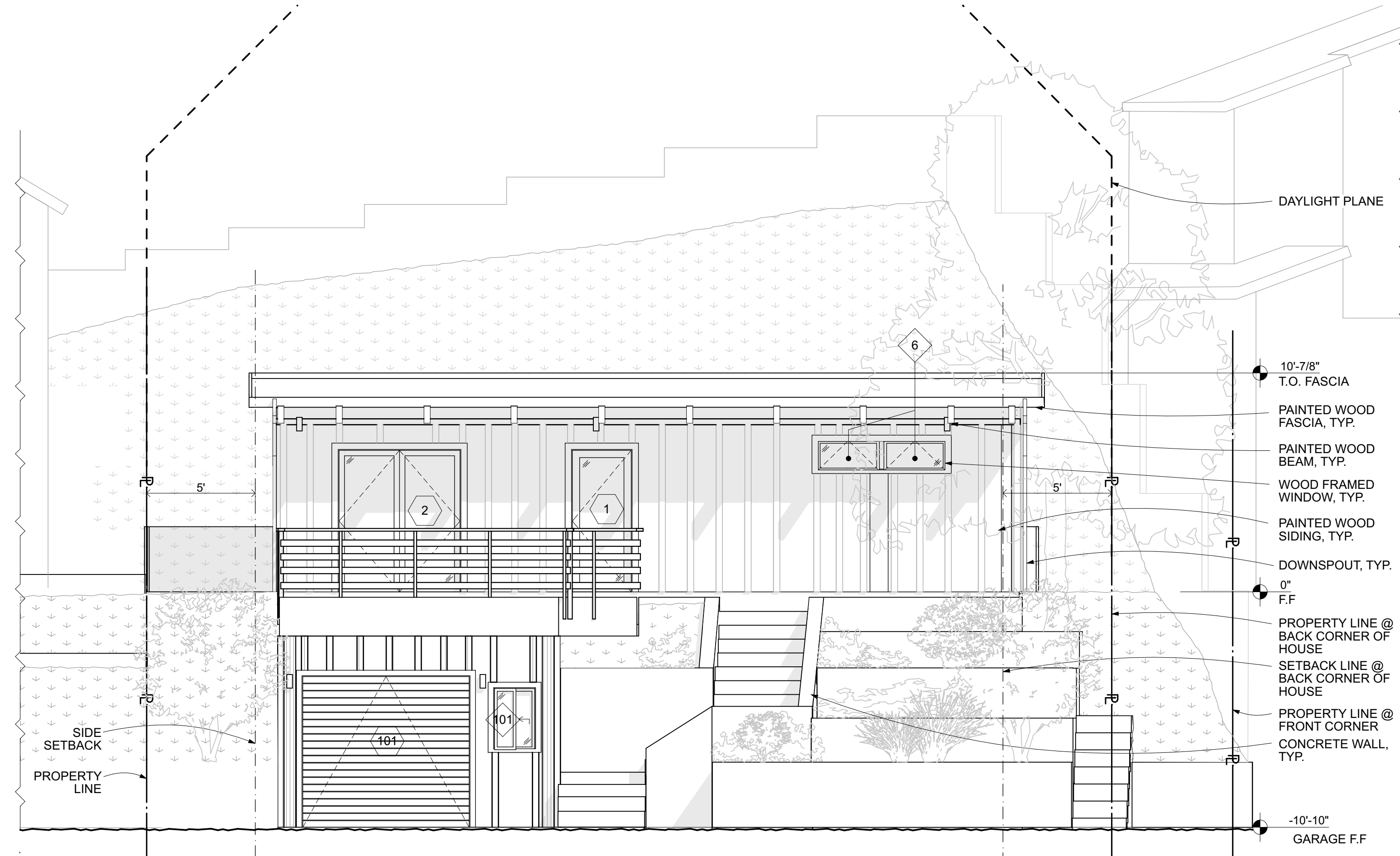
1 A2.0 EXISTING WEST SIDE ELEVATION SCALE: 1/4" = 1'-0"
